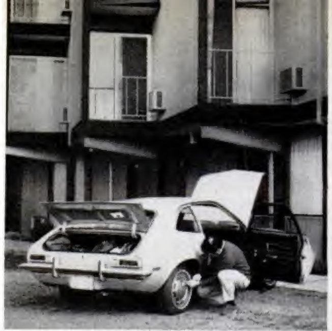
A MORNING RITUAL was checking tire air pressure. I ran the fronts and rears of both cars at 28 p.s.i.
